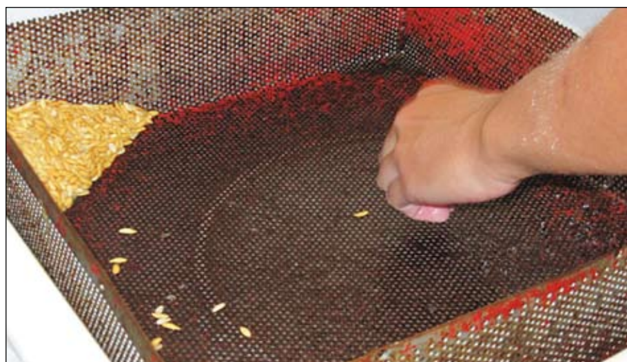
Hand melon seed cleaning screen at Hollar Seeds in Rocky Ford, Colorado.
